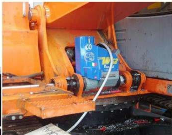
Restoring the supports of the chassis lift ram location without removing the cabin. Disassembling the cabin, on the new excavator machines, means that while reassembling it, there can be complications on the electronic and electrical apparatus.
