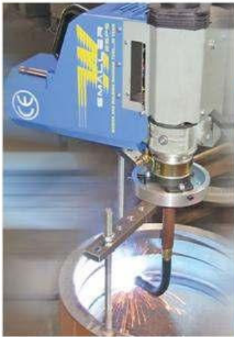
Overlay welding on \varnothing 380 mm
