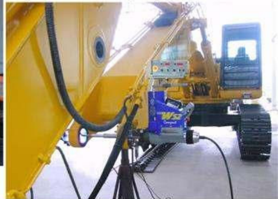
Reconditioning of the excavator arm. On-site operation, without disassembling the stick and the hydraulic tubes, while respecting the environment.
