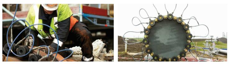
CTST tensioning tools are supplied with two hydraulic connections. This allows for very simple link hose configuration to link multiple bolt tensioning tools together.
