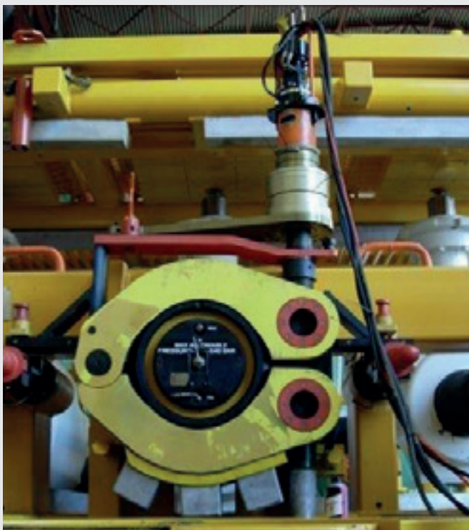
Wet Pipe Clamp Tool under test
