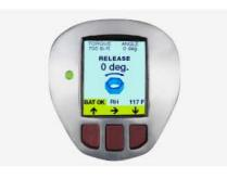
The LITHIUM SERIES makes torque and angle bolting simpler than ever before. The desired torque can be entered in Imperial or Metric, followed by the desired angle. When the trigger is pulled the tool will automatically apply the torque, pause, and then apply the programmed angle. When complete, the light on the back of the tool will turn green and a short beep will be heard.
