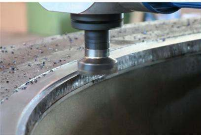
Tapping Operation M36X3
