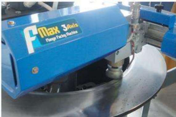
Surface facing finish on a flange coupling.
