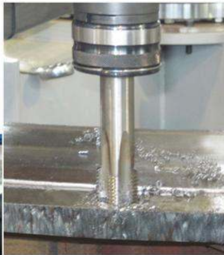
Tapping Operation M36X3
